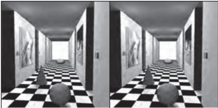
Fig. 9. Examples of stereo pairs of images (left and right) compressed with Markov Random Field algorithm
