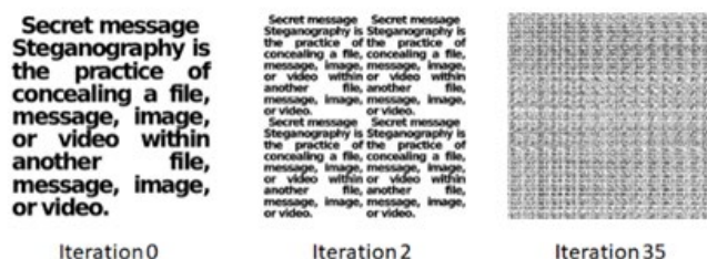
Fig. 4. Dynamics of hidden message transformations according to Baker's map up to 35 iterations
