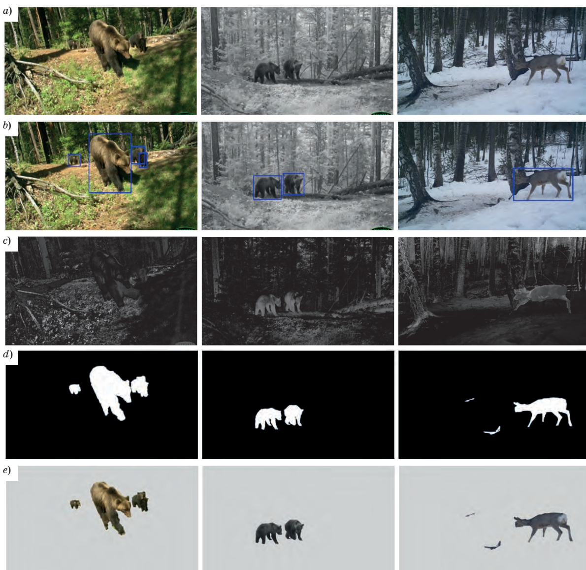
■ Fig. 5. Examples of segmentation and animal localization using Ergaki 2018 dataset: a — original images 2012_bear.jpg, 2017_IMG5044.jpg, and 2013_PICT1696.jpg; b — ground truth image segmentation; c — saliency detection; d — masks obtained from background and saliency estimation; e — results of localization
